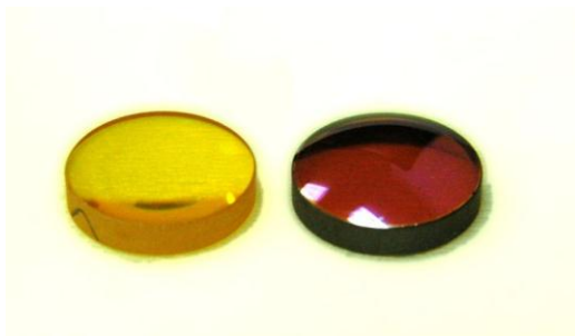
Fig. 2. ZnSe (left) and GaP (right) optical elements of bichromatic lenses for VIS and MWIR application
